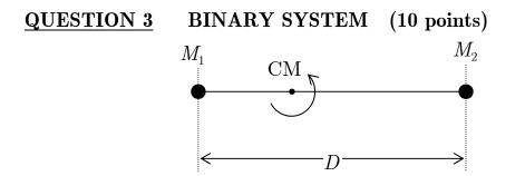
A binary star system consists of  $M_1$  and  $M_2$  separated by a distance D.  $M_1$ and  $M_2$  are revolving with an angular velocity  $\omega$  in circular orbits about their common centre of mass. Mass is continuously being transferred from one star to the other. This transfer of mass causes their orbital period and their separation to change slowly with time.
